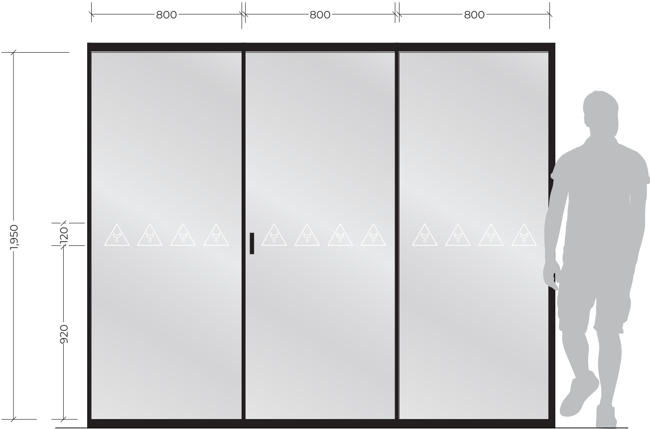
01 Sign 03: Store Room Glazing Elevation Qty x3 panels Scale 1:20
